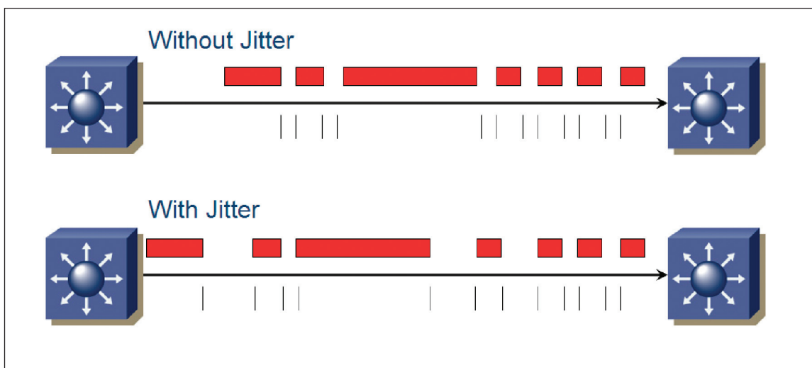
Figure 2. Packet transmission with and without jitter
